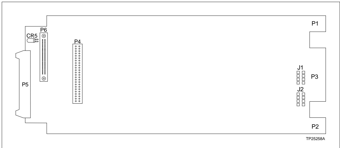
Figure 3-5. IMMPIO1 Module Jumper Locations
