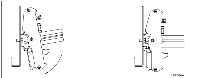
Figure PR3-1. Power System Assembly Installation
