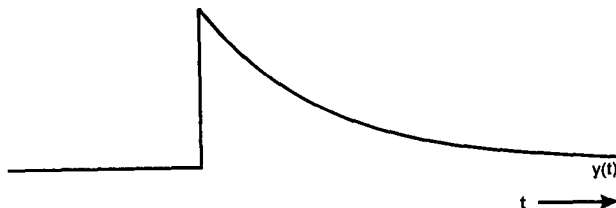
Fig 2-7 Impulse Response of a first order system
