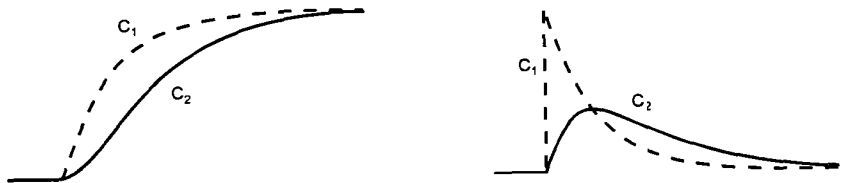
Fig 2-10 Stock consistency responses for two stock chests in series
