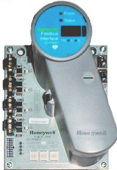
Figure 1 Series C FIM Mounted on non-redundant Input/Output Termination Assembly (IOTA).
